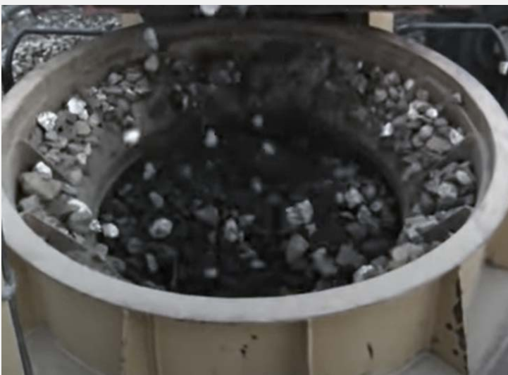
TRICKLE FEED Incorrect Method = Irregular Liner Wear
