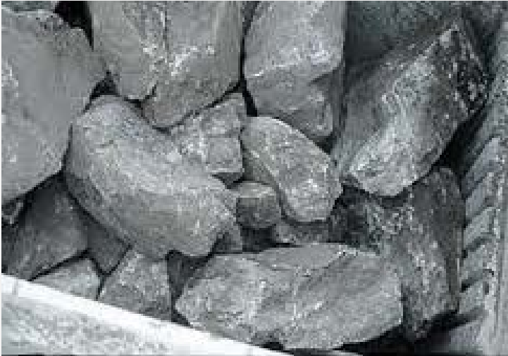
CHOKER FEED Correct Method = Uniform Liner Wear
